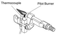
Figure 25 - Correct Pilot Flame Pattern
